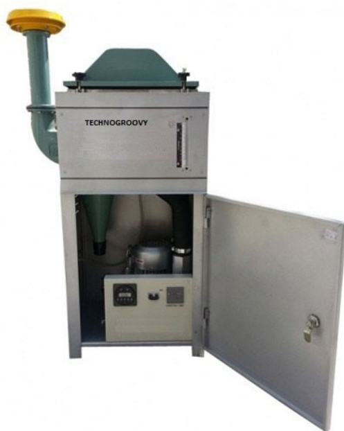
Figure 8.1: Typical high-volume air sampler
