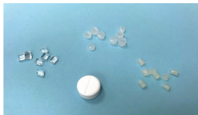
Figure 3.2.2. Examples of different types of plastic pellets and a pressed powder tablet used in the ILC.
